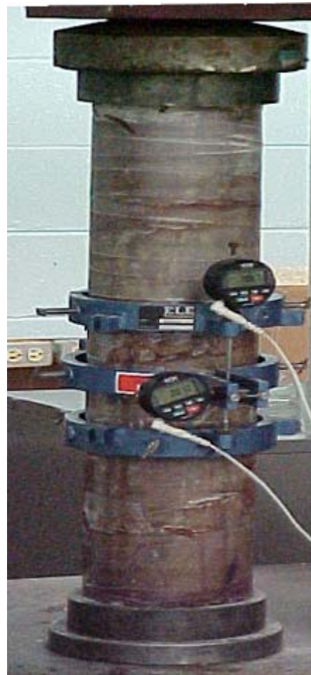
(b) Prepreg repaired sample
