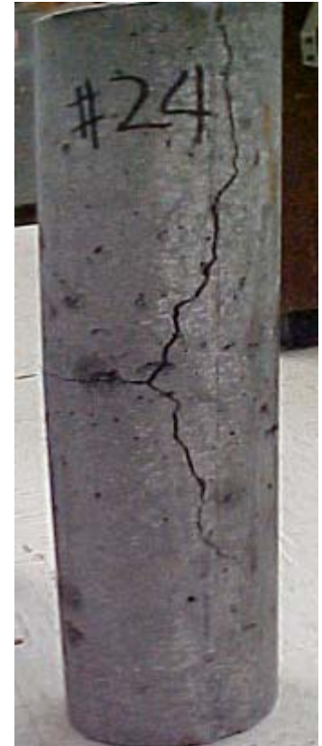
(b) Induced cracks
