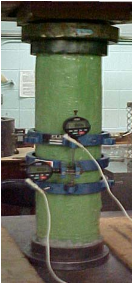
(a) Epoxy repaired sample
