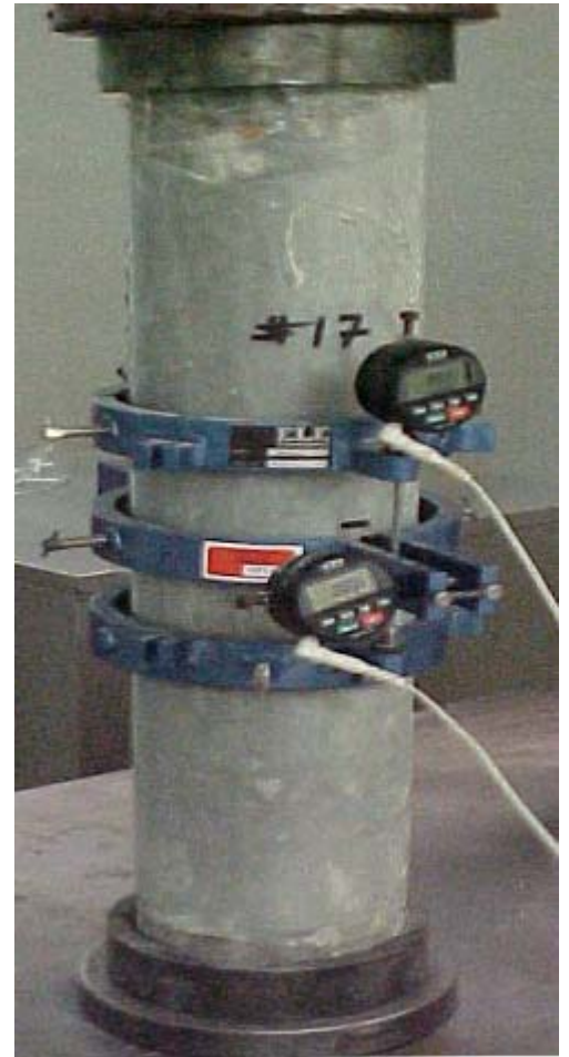
(c) UV curing resin repaired sample
