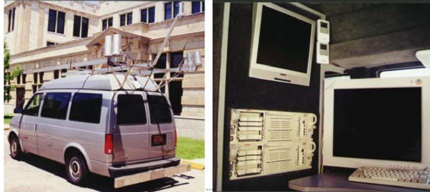
Fig.1. The original Digital Highway Data Vehicle (DHDV)
