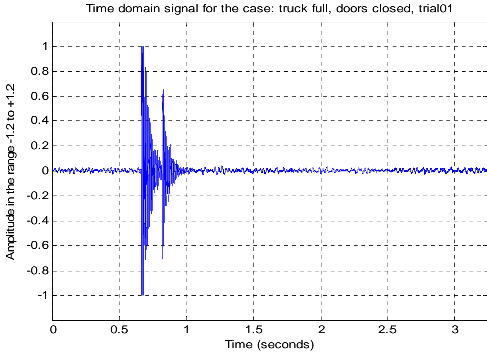
Figure 18: Echo sample for the case with trailer full doors closed.
